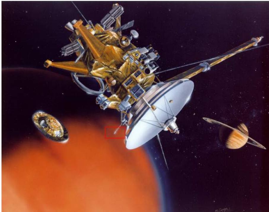
Figure 2.1: An artist's view of Cassini in orbit around Saturn releasing Huygens. The red rectangle indicates the location of the Langmuir Probe sensor, further discussed in section 5.1. Source: http://www.jpl.nasa.gov , September 12, 2007.
