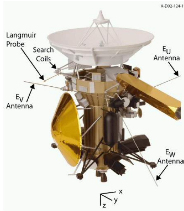
Figure 6.2: The picture shows the Cassini spacecraft and some of its instruments. The spacecraft axes are defined as shown in the bottom.
